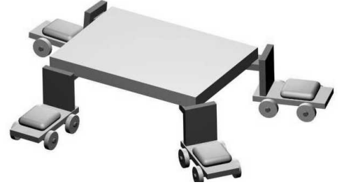
Figure 2. A group of robots lift a bulky object (note that there are four robots in this figure but we have used three robots in our simulations)
